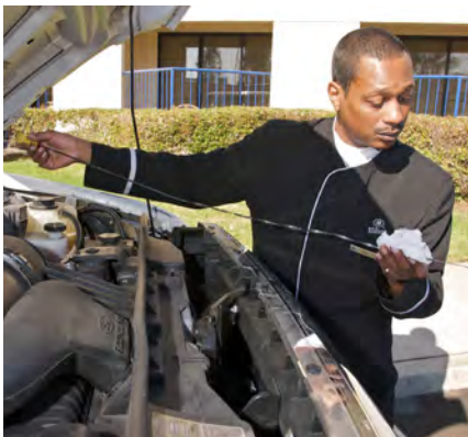
Look under the hood to check the fluid levels, including engine oil, coolant, brake fluids, etc.
