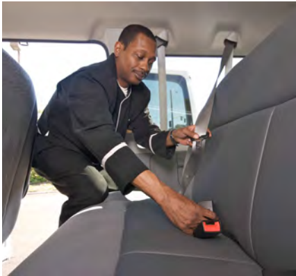
Check all installed seat belts to ensure they extend & retract easily and buckle securely.
